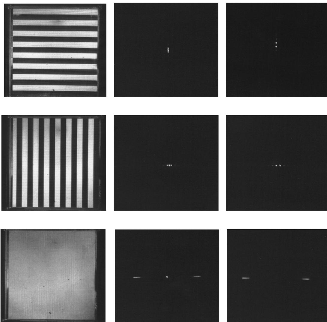
Figure 5. First column shows the SLM addressing; second column: far field diffraction pattern for a binary amplitude grating; third column: far field diffraction pattern for a binary phase grating.
