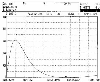
Figure 4. Transmission of PNLC film and Fresnel rhomb between parallel polarizers.
