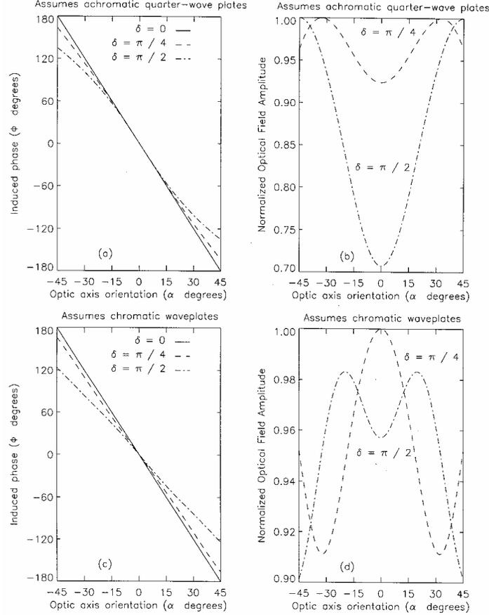
Figure 3. Complex transmittance of QHHQ. (a) and (b) phase and amplitude for the case of achromatic quarter-wave plates. (c) and (d) phase and amplitude assuming all chromatic elements.
