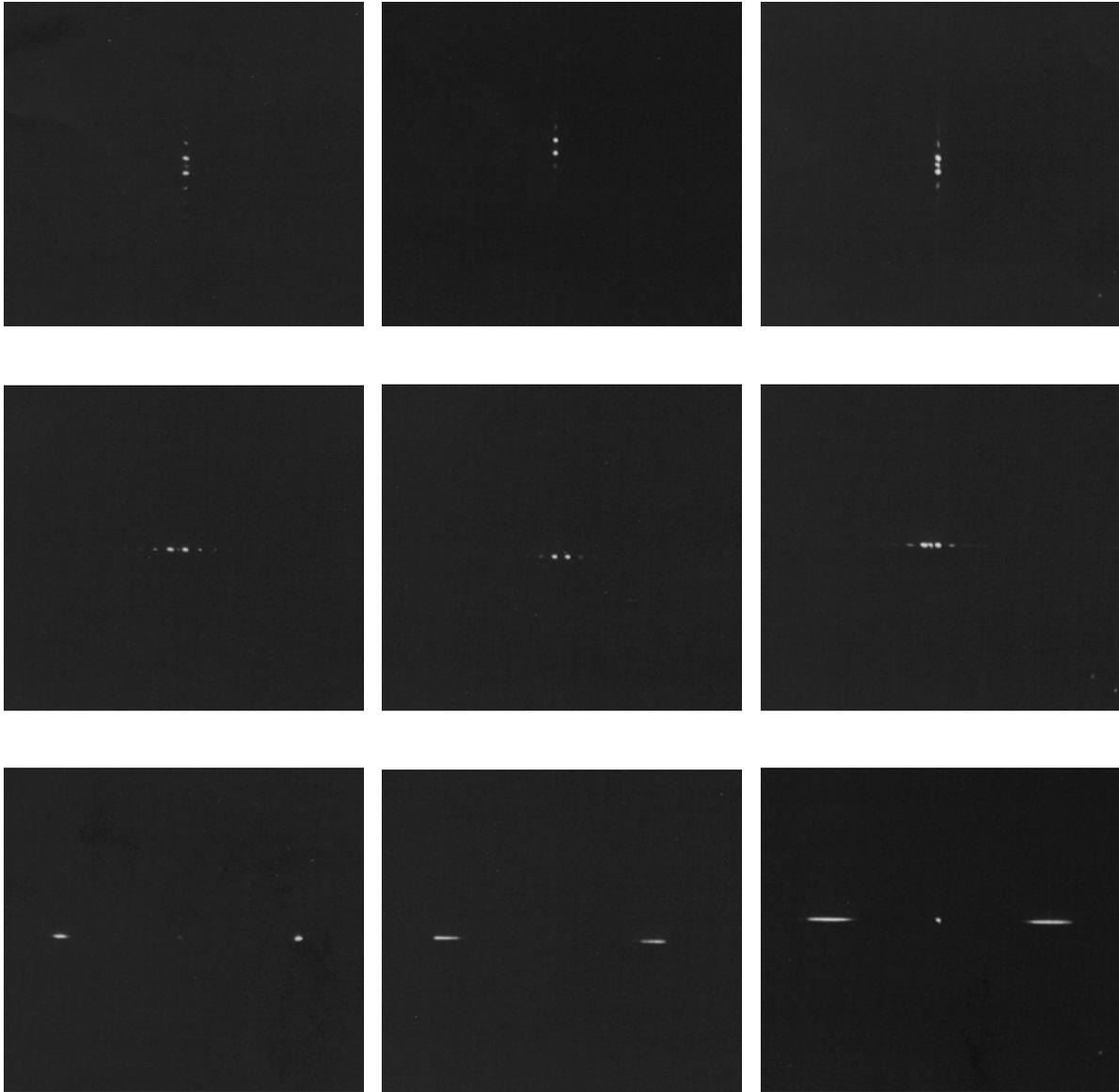
Figure 6. Diffraction patterns for binary phase written to the SLM, first column, monochromatic light (685 nm); second column, white light (400 nm to 650 nm); third column, white light, (400 nm to 1100 nm). Each row corresponds to the pattern in the same row of the first column in the previous figure (Figure 5).
