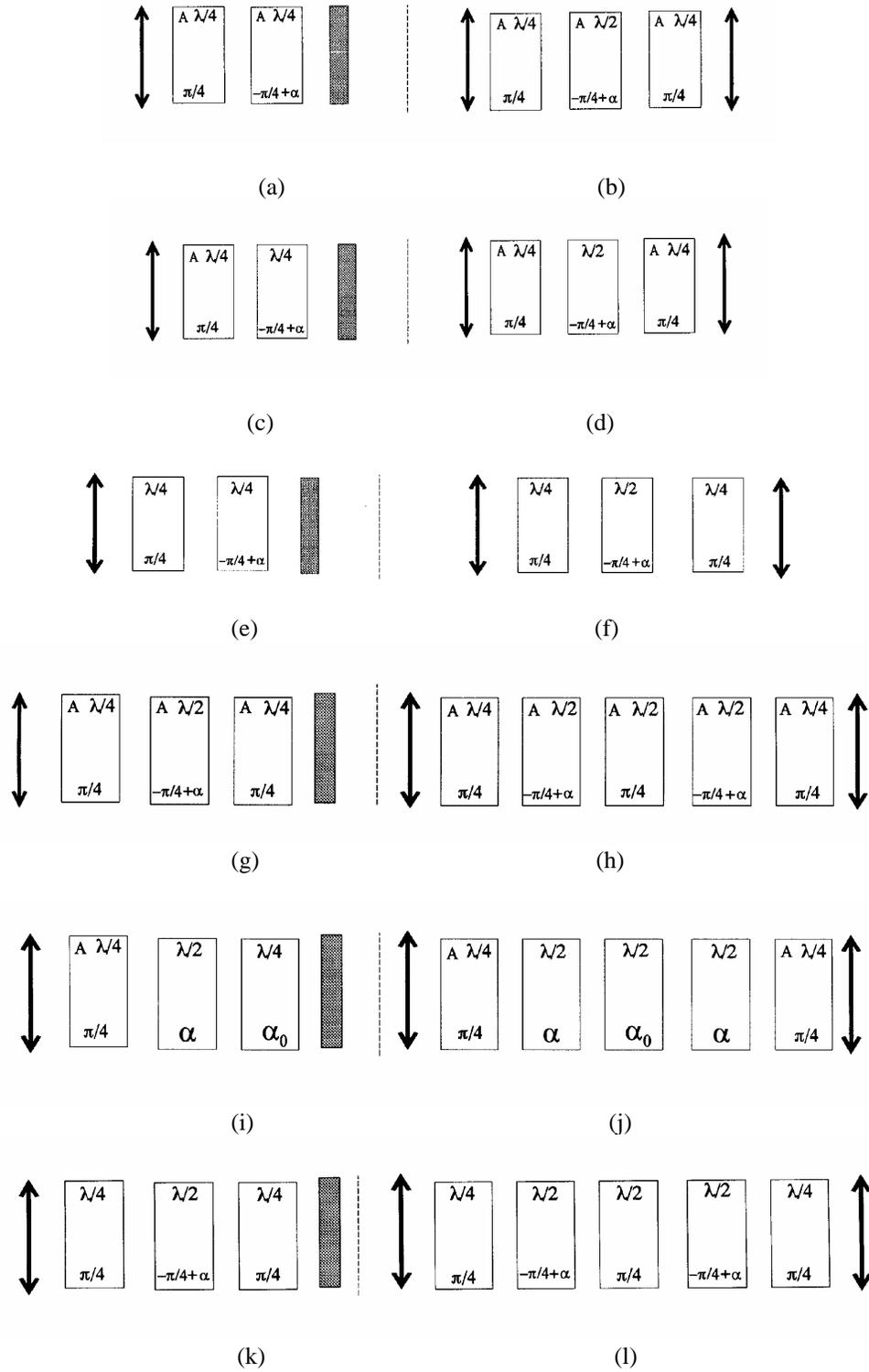
Figure 2. Reflection mode and unfolded phase shifter designs. (a) and (b) achromatic QHQ; (c) and (d) QHQ with a chromatic half-wave plate; (e) and (f) chromatic QHQ; (g) and (h) achromatic QHHQ; (i) and (j) QHHQ with chromatic half-wave plate, (k) and (l) QHHQ with all chromatic elements.
