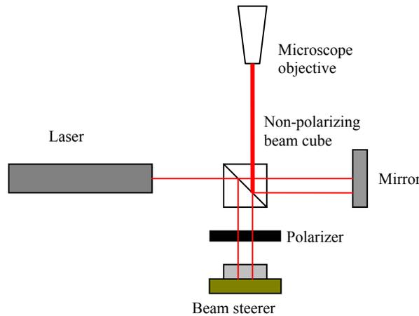
**Figure 1.** Schematic of the Michelson interferometer set-up used to measure phase modulation depth for normal incidence.
