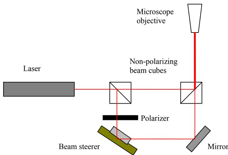
**Figure 2.** Schematic of the Mach-Zehnder interferometer used to measure the phase modulation depth for oblique incidence.
