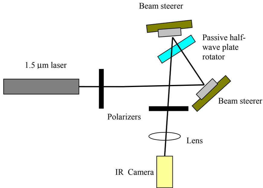
**Figure 3.** A schematic showing the set-up used for the two-dimensional beam steering demonstration.
