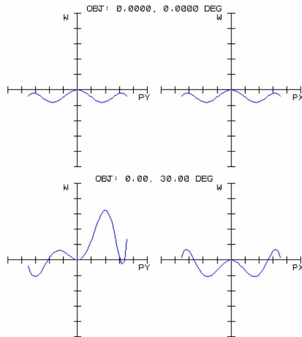
Figure 3: Wavefront error with SLM correction at the 0° and 30° fields as a function of normalized pupil (maximum scale is  $\pm 0.25\lambda$ ).
