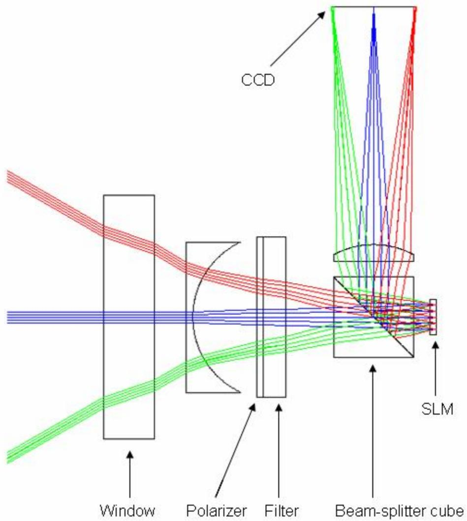
Figure 1: Optical layout of the final design (EFL = 27mm,  $f/7.7$ , FOV = 60°).
