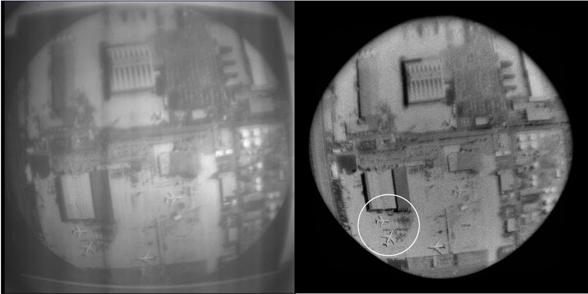
Figure 5: Image with the SLM correction applied to resolve the two planes at the left-bottom.
