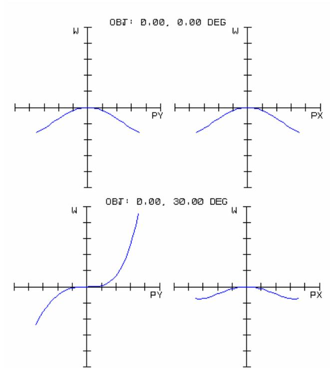
Figure 2: Wavefront error (OPD versus normalized pupil) without SLM correction at the 0° and 30° fields as a function of normalized pupil (maximum scale is  $\pm 25\lambda$ ).
