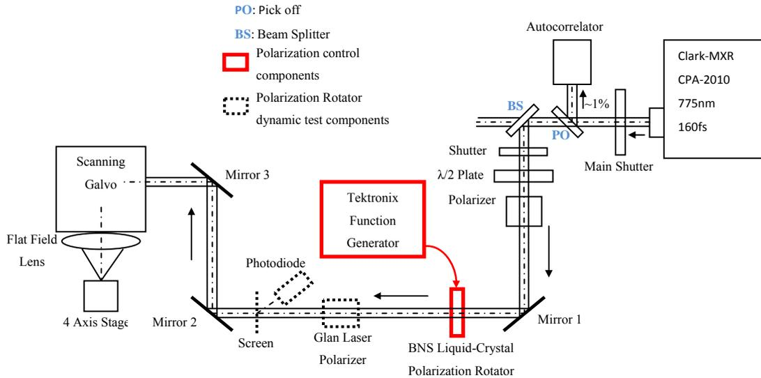
**Fig. 1.** Helical drilling experimental setup showing how the liquid-crystal polarization rotator was used. For the drilling tests, the dashed components were removed. This setup is a modified version of the one used in [11].
