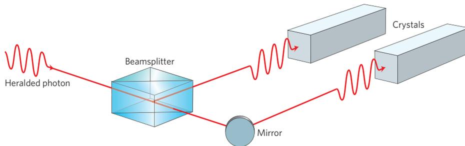
**Figure 2** | Creating entanglement between two quantum memories. A heralded single photon (the ‘pea’) first passes through a beamsplitter. The outputs of the beamsplitter are directed to the two crystals (the ‘shells’), where the photon is absorbed to produce a single excitation. The lack of information regarding the path of the photon creates an entangled state between the two crystals.
