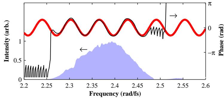
Fig. 3. Verification of phase calibration by applying a low-frequency sinusoidal spectral phase. Spectral intensity (light blue patch), applied phase mask (red line), and phase as measured by spectral interferometry (black line).
