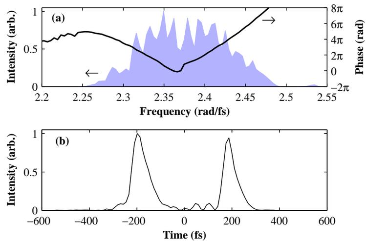
Fig. 4. (a) Measured spectral intensity (light blue patch) and phase (black line) for splitting a pulse into a delayed pair. (b) Temporal intensity, showing separation of 400 fs.
