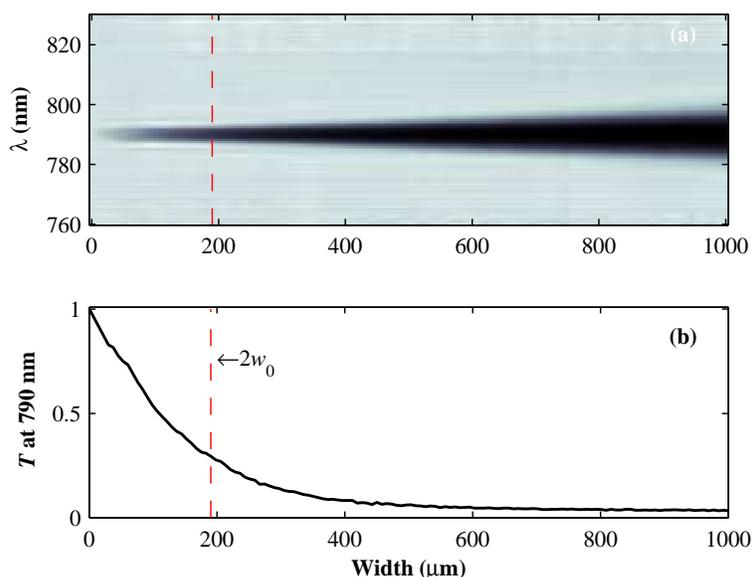
Fig. 5. Spectral notch of increasing width. (a) Measured spectra, normalized by the first spectrum, showing increased attenuation and broadening of notch as phase grating width is increased. (b) Transmission  $T$  at 790 nm, showing increase in attenuation which levels off when the phase grating is wider than the spectral focus  $2w_0$ , marked by the red dashed line.
