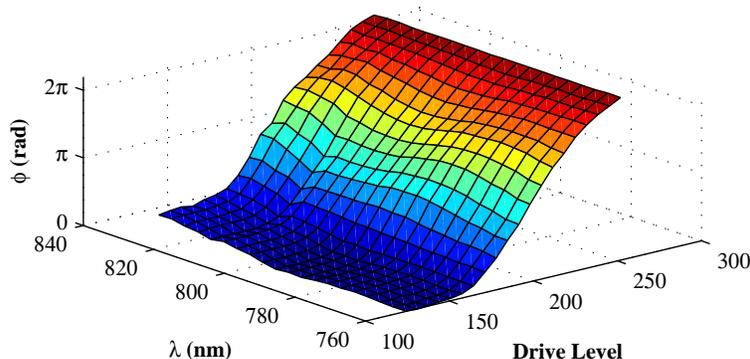
Fig. 1. Calibration of phase  $\phi$  with respect to wavelength  $\lambda$  and drive level. Surface mesh lines are shown to enhance visualization of surface curvature; actual data is collected at higher resolution.
