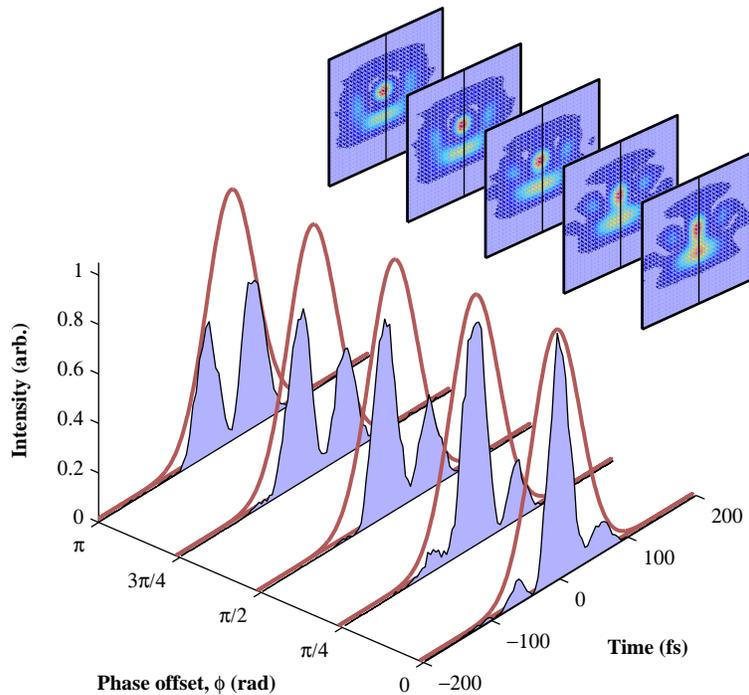
Fig. 7. Temporal profiles for the spectral double-slit experiment. Inset: FROG traces depict both measured (left half of trace) and numerically reconstructed (right half) traces.
