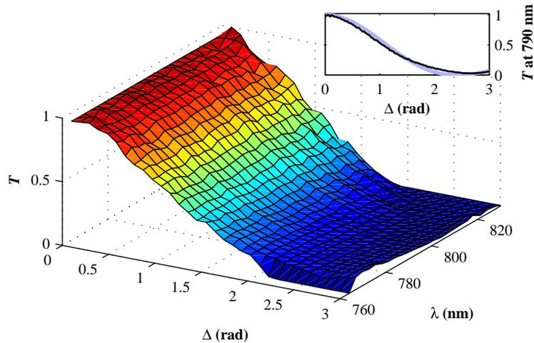
Fig. 2. Measured transmission  $T$ , plotted with respect to increasing phase grating depth  $\Delta$ , as applied across the entire phase mask. Surface mesh lines are shown to enhance visualization of surface curvature; actual data is collected at higher resolution. Inset: line-out of the above plot at 790 nm, showing transmission  $T$  with respect to the phase grating depth (black line). Theoretical curve (light blue line) shown for comparison.
