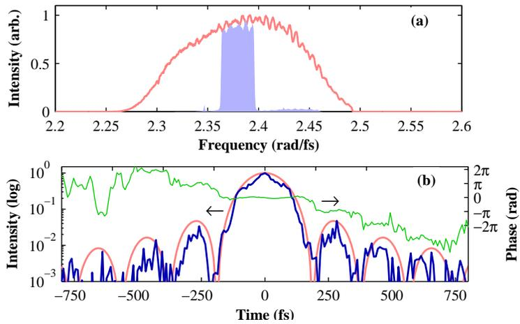
Fig. 6. Amplitude-only shaping. (a) Unshaped (red line) and shaped (light blue patch) square spectrum. (b) Resulting temporal profile (blue line), with a sinc<sup>2</sup> (red line) for comparison. Spectral phase (green line) shows  $\pi$  phase offset between adjacent lobes.
