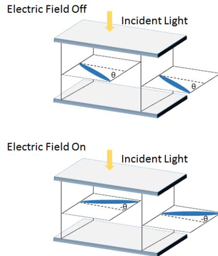
Nematic (left) and Ferroelectric (right) liquid crystal operation. Nematic liquid crystal provides analog phase modulation through out-of-plane rotation and modulation of the effective retardance. Ferroelectric liquid crystal provides switchable in-plane rotation of the optical axis for polarization rotation at fixed retardance.
