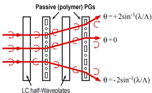
A two-stage LCPG beam steering module. In the top ray, the second switch is active and the ray is steered in the positive direction. In the bottom ray, the first switch is active and the ray is steered in the negative direction. When both switches are off, the ray is unaffected.
